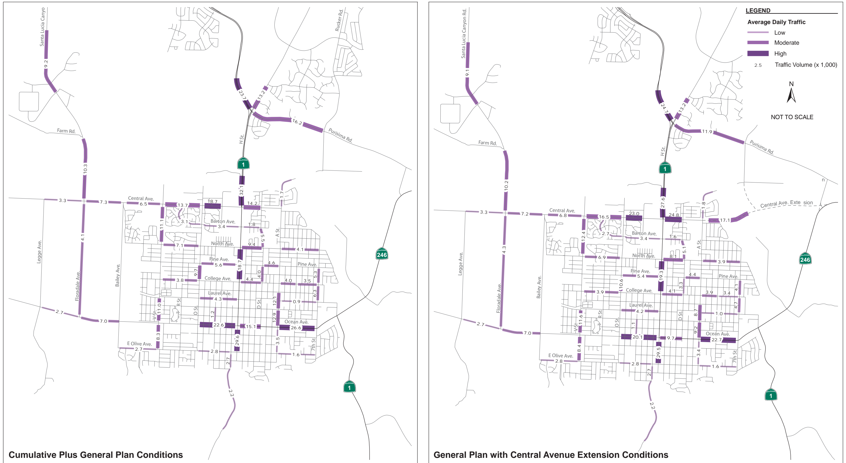
Cumulative plus General Plan and General Plan with Central Avenue Extension Average Daily Traffic Volumes
